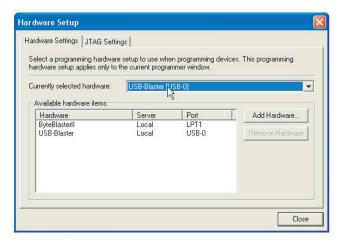
4. Click **Auto Detect** to verify correct setup and to display the MAX II and Stratix II GX devices in the JTAG chain (Figure A–5). You may have to press the **CONFIG** switch, S1, on the board during this process before the flash chip appears in the chain.
