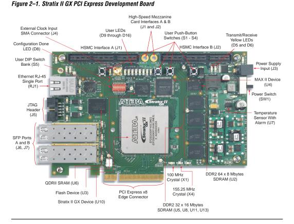
Figure 2–1 shows the Stratix II GX PCI Express development board.
