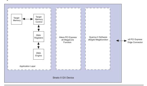
Figure 2-3. Stratix II GX Device Block
