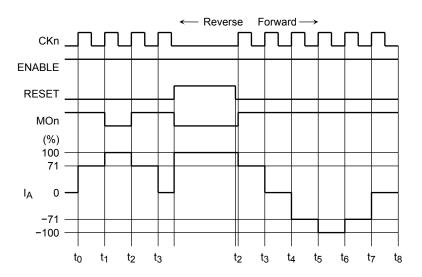
Setting the RESET signal High causes the outputs to be put in the Initial state and the MOn output to be driven Low.
