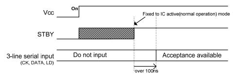
Input the Serial Signal (3-line) after waiting over 100ns period from the STBY fixed to "H", that means IC normal operation starts.
