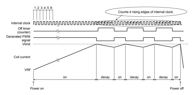
(The upper limit of the coil current (IO peak) can be calculated as: IO = Vlimit/RNF.)
