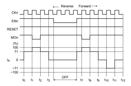
Setting the ENn signal Low disables only the output block, and the internal circuitry continues to operate in accordance with the CKn input. Therefore, when the ENn signal is set High again, the output current restarts as if phases had proceeded with the CKn signal.
