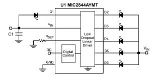
LCD Display Backlight with Six WLEDs
