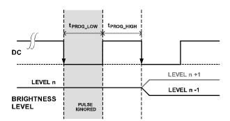
Figure 10. Brightness Programming Pulses
