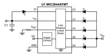
Figure 3. High Current LED Driver Circuit
