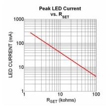
Figure 2. Peak LED Current vs. R<sub>SET</sub>
