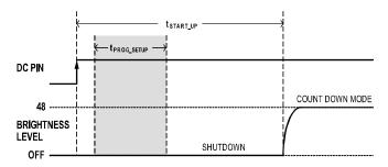
Figure 6. Typical Start-Up Timing
