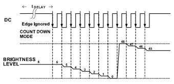
Figure 12. Down Counter Roll-Over
