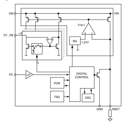
Figure 1. MIC2844A Functional Block Diagram
