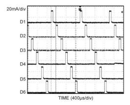
Figure 5. LED Current 60° Phase Shift
