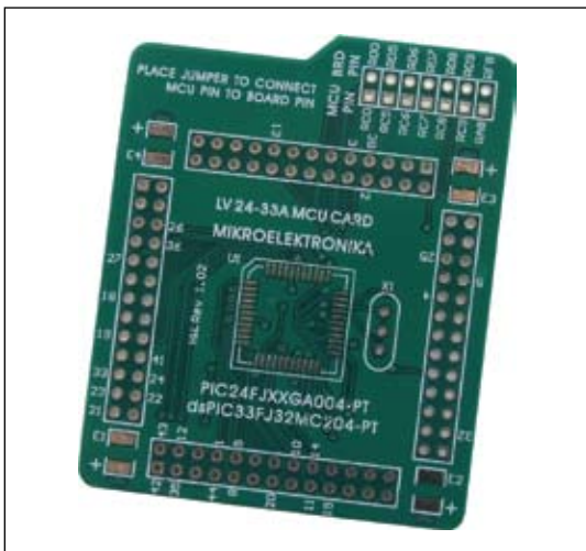
Figure 35: Empty MCU card MCU Card 12
